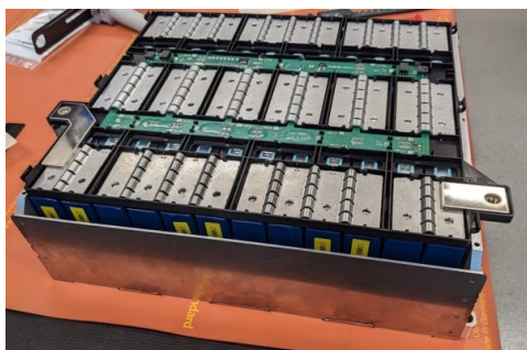
Figure 7 Manufactured cell-stack assembly.
