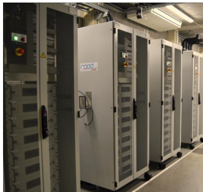
Figure 13: Testbench to validate the battery pack
