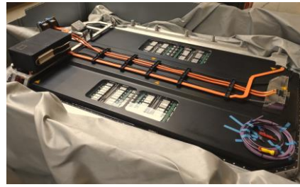
Figure 12: Assembled LIBERTY battery pack
