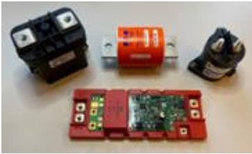
Figure 2: Semiconductor based battery main switch compared to replaced component
